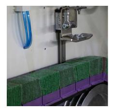
\_\_ 2 counterrotating cross-belts with automatic abrasive wear compensation
