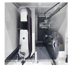
deburring and edge rounding with an abrasive contact roller and cross belt system
