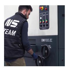
the compact size takes less floor space and it's easier to operate while delivering the same top-quality deburring and edge rounding
