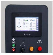
\_\_touchscreen control panel for automated and motorized adjustments with machine statistics and errors
