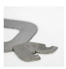
\_\_ grinding laser burrs and rounding the edges in one single step: high performance on all edges and also on internal holes
