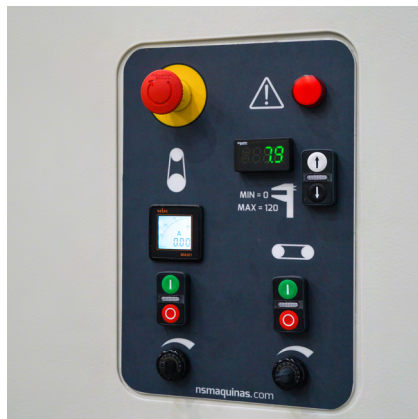
__ simple and intuitive control panel with motorized thickness adjustment buttons
