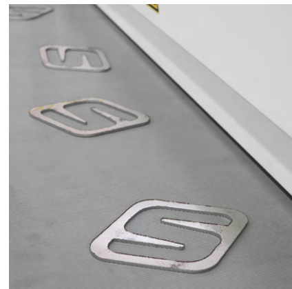
__ it allows surface finishing on metal sheets up to 1600mm width and as small as 50x50mm metal parts
